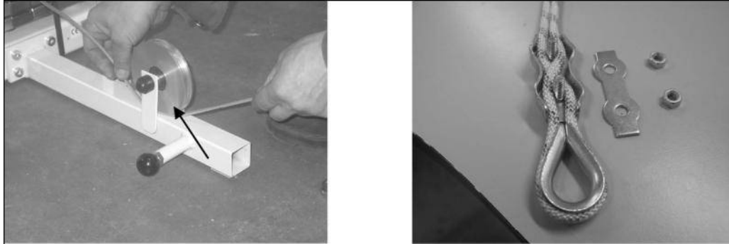
Figure 10: a) Triangle sticker downwards b) Locking the rope
